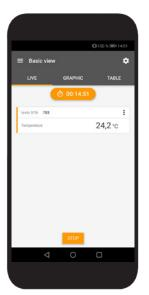
The cost-free testo Smart App turns your smartphone/tablet into the display for the testo 915i. The operation of the Smart Probe and the display of the measurement values take place wirelessly by Bluetooth® on your smartphone – independently of the measurement location. In addition, you can use the App to create measurement reports, add photos and comments to these and conveniently send them by e-mail.
