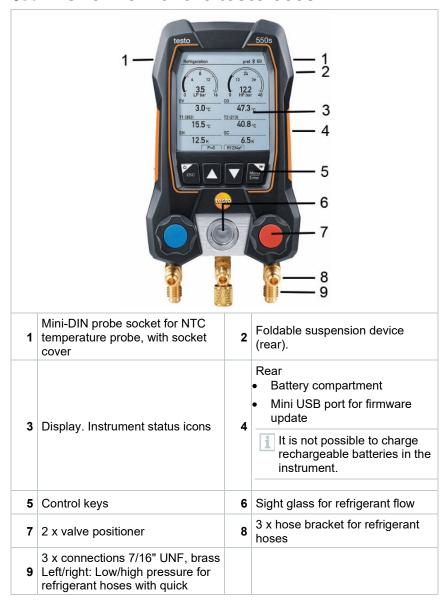
release screw fitting; passage can be closed via valve positioner Centre: e.g. for refrigerant bottles, with sealing cap, refrigerant hoses with quick-release screw fitting; passage can be closed via valve positioner.
