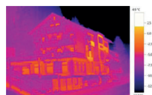
Thermal image with ScaleAssist
